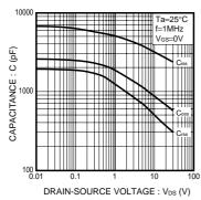
Fig.1 Typical Capacitance vs. Drain-Source Voltage
