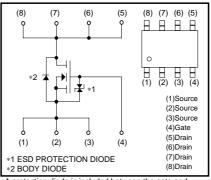
\*A protection diode is included between the gate and the source terminals to protect the diode against static electricity when the product is in use. Use the protection circuit when the fixed voltages are exceeded.
