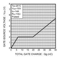
Fig.3 Dynamic Input Characteristics
