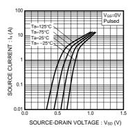
Fig.6 Source Current vs. Source-Drain Voltage
