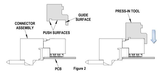
3. Using the application tool and an appropriate press, seat the Orthogonal Direct Ram module until there is less than 0.10mm (.004in) clearance between the bottom of the plastic housing and the surface of the PCB. See Figure 3.
