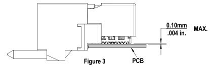
There should be no broken stand-offs along the perimeter of the part (an indication of over-pressing).
