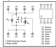
A protection diode is included between the gate and the source terminals to protect the diode against static electricity when the product is in use.Use a protection circuit when the fixed voltage are exceeded.
