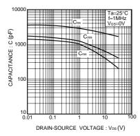
Fig.1 Typical Capacitance vs. Drain-Source Voltage
