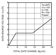
Fig.3 Dynamic Input Characteristics
