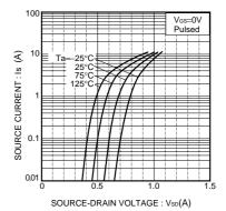
Fig.6 Source-Current vs. Source-Drain Voltage
