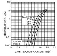
Fig.4 Typical Transfer Characteristics
