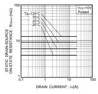
Fig.7 Static Drain-Source On-State Resistance vs. Drain Current (1)
