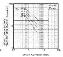
Fig.7 Static Drain-Source On-State Resistance vs. Drain Current (3)
