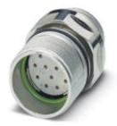
Device connector for front wall, straight, shielded: yes, SPEEDCON locking, M23, No. of pos.: 12, type of contact: Socket, Solder connection, Axial seal, Central fastening M20 x 1.5, can be positioned via a locking put
